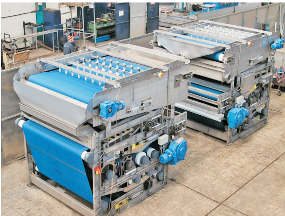
Combined Belt Units during manufacturing
